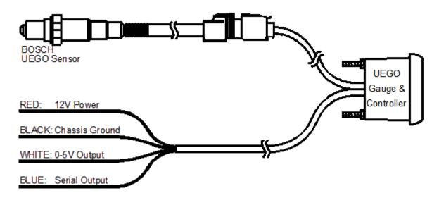
Figure 3. Gauge Installation Connections
