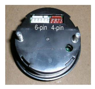
Figure 4. Gauge Side Harness Connections
