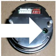
Figure 10. Calibration position screw location
