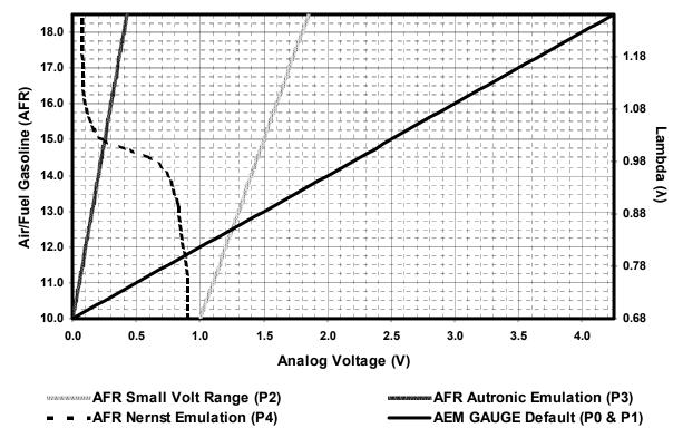
Figure 9. Calibration graph of available outputs
